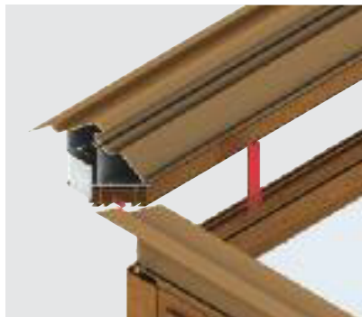
Fix ringbeam to existing windows
